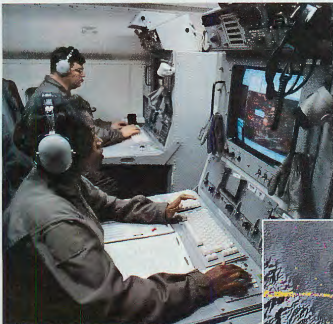
(above) Monitoring ground movements in Kosovo at one of the onboard J-STAR computer work stations. (right) Enemy armor assets are depicted on the J-STAR screen as yellow dots. Vehicles are shown as purple dots.
